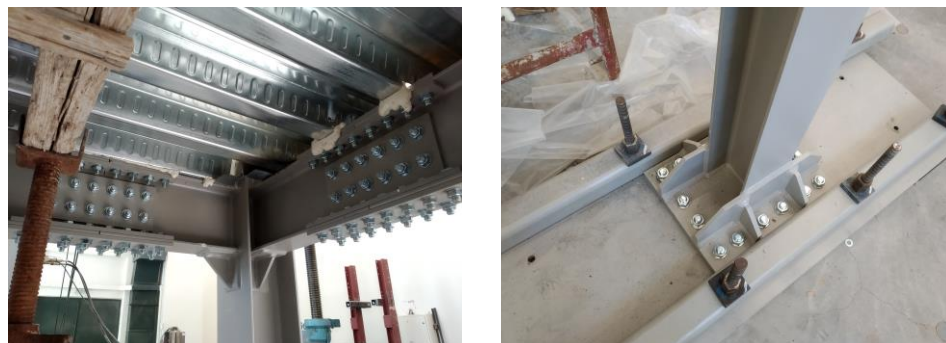
Figure 2: Detailing at the beam-column joints (left) and column base (right) of the test frame.
